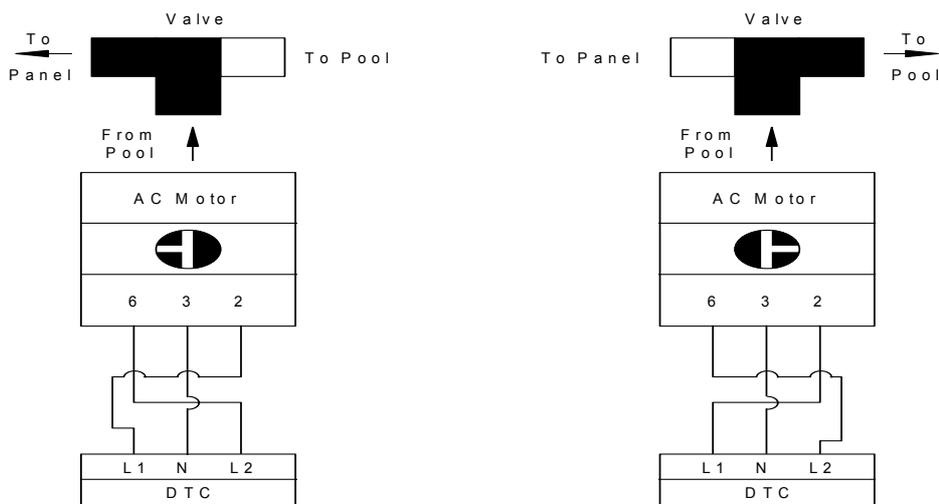
Solar heat gain L1 - 2 live      No solar heat gain L2 - 6 live
