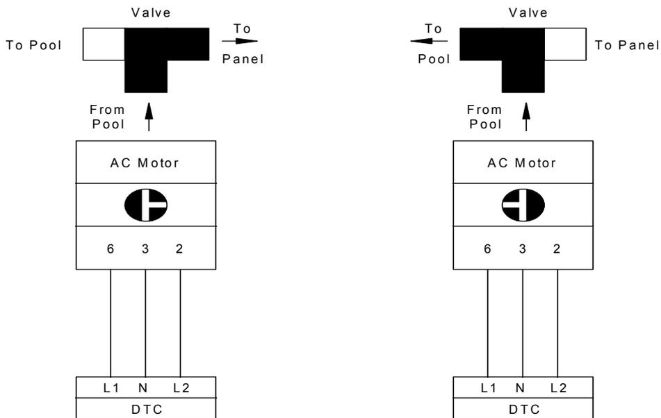
When it is necessary to plumb the outlet pipes to pool and panels into opposite valve ports reverse L1 and L2 as follows:
