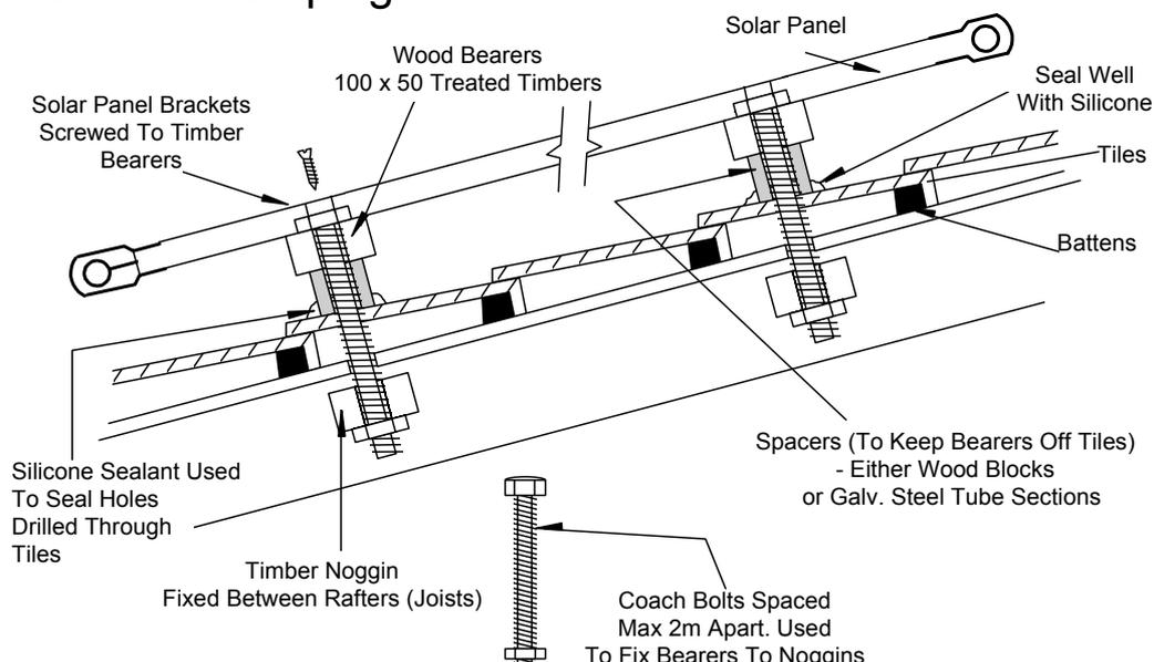
Mounting the framed panels (Models 030 and 020) on the roof is relatively simple since the two bearers must be at the same distance apart as the top and bottom fixing brackets on the panels.
