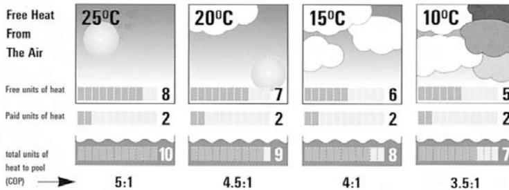
Sunshine is not essential for this system as all it needs is air; A heat pump can work with air temperatures as low as -15 degrees centigrade (dependent on the model chosen) and then becomes more efficient as the temperature increases.
