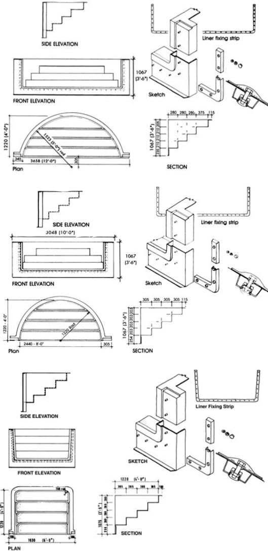
*Note:* Step Unit dimensions can vary, please check with All Swim prior to installation if step unit is not on site.
