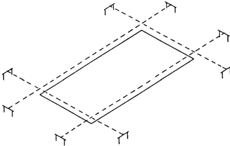
*The four corner pegs of the pool must form a rectangle with the diagonals equal.*
