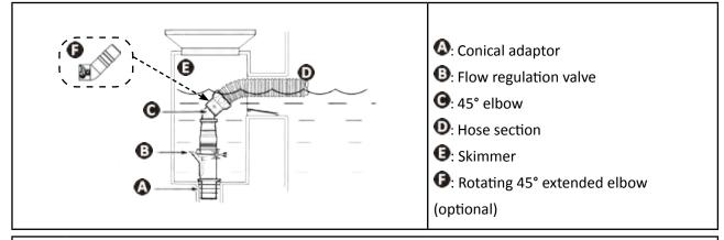
Tip: Protect the filtration system by connecting the flow regulation valve This valve is used to adjust the flow to optimise the cleaner's performance; it is also very useful for retaining any debris that may be sucked in and damage the filtration equipment.
