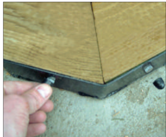
STEP 4 - Screw the 6mm coach screws into the outside of the steel corner plates. Cover the screw head with the plastic caps. Drill 4mm pilot holes if needed.
