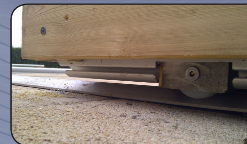
• Brake with rubber pad and guide wheel
