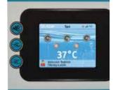
Press () jet button a second time to place the hydromassage jets in a high speed, you will see the jet 1 icon on the screen rotate faster.
