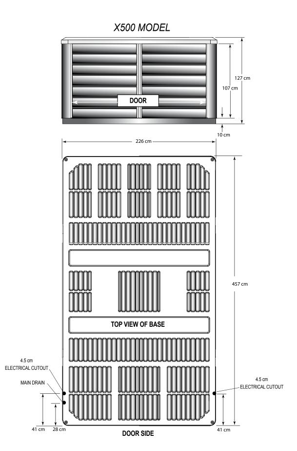
NOTE: ENDLESS POOLS requires that the X500 Model be installed on a minimum 15 cm (6") thick reinforced concrete pad or structurally sound deck able to support the "dead weight" found in the specification chart on the back page.
