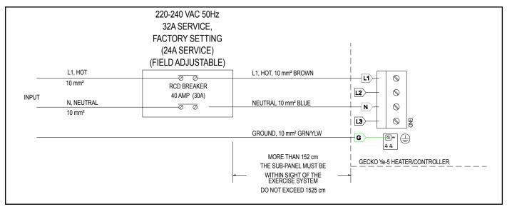
IMPORTANT: Using a 24A service will require a system modification, see Electrical Configuration on page 14 on how to change the system settings.
