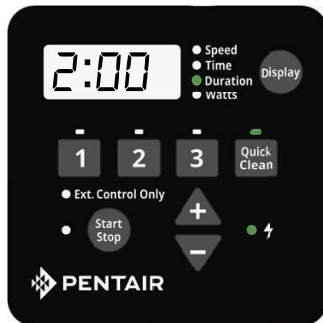
Figure 13: Setting Duration for Quick Clean
