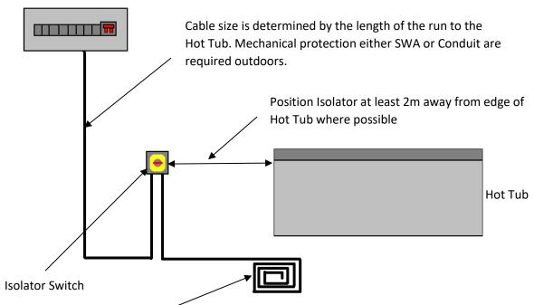
Please leave 4m of coiled wire by the side (nearest to the Isolator) of where the Spa will be positioned. This will allow you to choose the final position of the Spa on the day and not be restricted by the length of cable. Please also identify Live Neutral and Earth on harmonised colours. Please also leave a suitable gland kit with cable.
