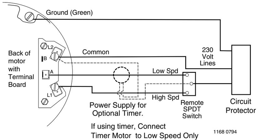
**Figure 4C – Wiring hook-up diagram, two speed motors.**
