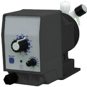
An economy solenoid driven **pulse proportional** dosing pump with manual stroke length adjustment plus a **low level probe**. This pump, similar to the VCL, will automatically stop dosing once the chemical in the storage container reaches the low level.
