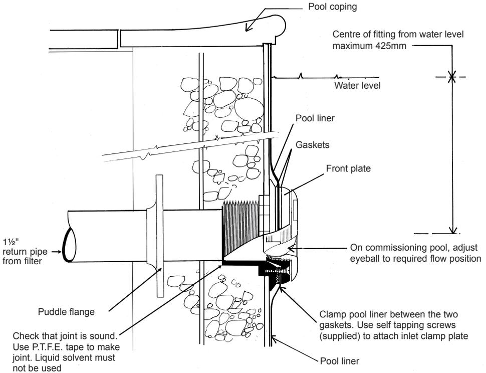
**IMPORTANT: all pipework and pool fittings must be pressure tested before backfilling and commissioning**
