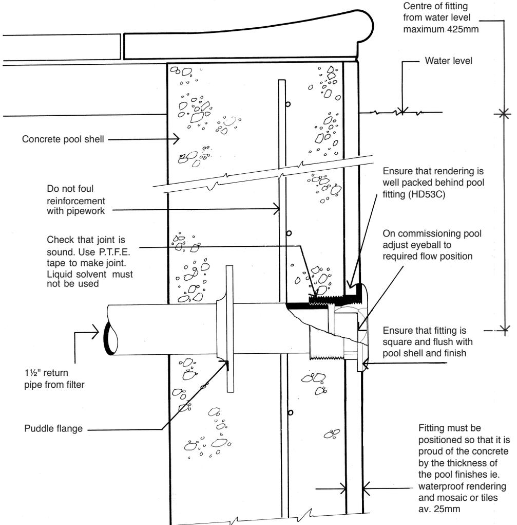
**IMPORTANT: all pipework and pool fittings must be pressure tested before backfilling and commissioning**
