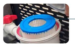
When replacing the filter element, please close the water inlet and outlet valves of the tub, loosen the filter exhaust valve by counter clockwise, then unscrew the filter cover, remove the filter element, and replace the filter element.
