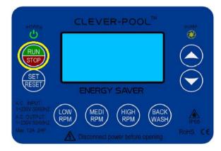
To stop the pump simply press the RUN/STOP button again.
