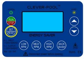
Press the BACKWASH button. The display will now show backwash and the rpm.
