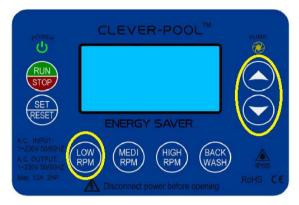
Press the RUN/STOP button to put it into run mode, this will start the pump. When the chlorinator timer turns off, the CLEVER-POOL will store the speed and resume at that speed when switched on again.
