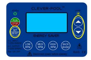
Press the SET/RESET button to store the speed and step over to AUTO MODE 2. The display should show CURRENT TIME, START TIME, STOP TIME and the stored time with hours digits flashing. This is the start time for AUTO MODE 2.
