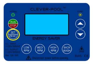
Press the SET/RESET button to store the time. The display will now show the current time with flashing cursor and the word shown at the top.
