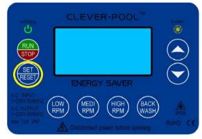
Press the SET/RESET button to step to SPEED setting. The display will now show the flashing four digits for speed, which is the speed for AUTO MODE 1. Press the up or down button to change motor speed. Alternatively press one of the systems preset speed buttons LOW RPM, MEDI RPM, HIGH RPM.
