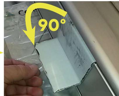
Rotate the bracket down
