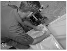
Attaching The Cover & Bonding Wire
