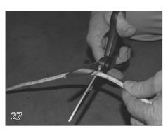
Pull both ropes until the leading edge just moves on each side, cut the longer rope to the same length as the shorter rope while tight. These ropes should be at least 8ft long. Use a lighter or torch to burn the ends of the rope. In most cases you will only need to cut one rope.
