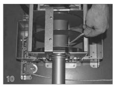
Direct this rope under the rope reel, over the rope containment bracket and out of the mechanism.
