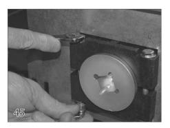
The roll up tube brake on the non motor end should be tight enough to prevent the cover from rolling off the tube faster than it is being pulled into the track. To adjust this brake, use two 7/16" wrenches and tightening or loosening the thru bolts in the brake block.
