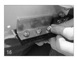
Attach the detachable rope tab to the three hole plate on the wheel assembly.
