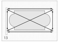
Lengths, widths and diagonal dimensions <u>must</u> be equal to each other or the system will not operate properly.
