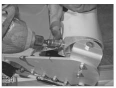
Connect the bonding wire that is attached to the front corner of the cover to the leading edge bar using a tek screw. Be sure the screw doesn't interfere with the leading edge insert.
