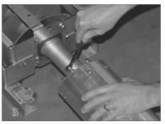
With the motor end turned upside down, attach the cone one the motor end using the same bolts (28) and lock washers (23). Tighten the bolts with a 9/16" wrench.
