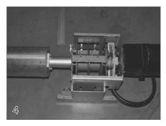
Positioning the Mechanism Place the mechanism on the pool deck roughly in the position that it will be anchored.
