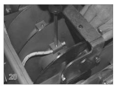
Attaching The Ropes to the Rope Reel Loosen the set screw and remove plastic plug from the rope holder tube. Bring the ropes back to the mechanism. Attach the ropes to the rope reel by inserting the ropes through the center of the rope holding tube and tighten the set screws firmly into the ropes. Some prefer to tie a knot at the end of the rope.
