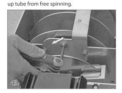
To loosen the brake, use an allen wrench to turn the set screw inside the jam nut in the counter clockwise direction.
