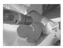
Position the fabric on the leading edge so it is in line with the leading edge support bracket. Secure with a tek screw (24) on the back side of the leading edge. Be sure the screw does not interfere with the leading edge insert.
