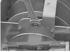
If you need to adjust the rope reel brake, first loosen the jamb nut on the side of the rope reel mechanism.
