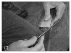
File the track ends on both sides of the pool making sure to round all edges and remove all burrs. This step is extremely important. The cover can damaged very easily by metal burrs and this damage is not covered by the warranty.
