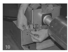
Use a 7/16" wrench to tighten the nylock nuts. Additional carriage bolts (27) and nylock nuts (29) are provided and can be used as reinforcement for the pulley brackets as needed.
