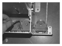
Routing the Ropes Begin with the rope on the motor end. Feed the wire that is attached to the rope around the first and second pulleys.
