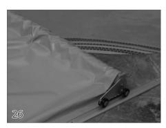
Pull the cover back until the cover is in the tracks equally on both sides. Pull the ropes tight as they come off the pulleys on the mechanism to eliminate the slack in the rope.
