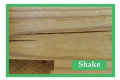
**Shake** appears like a series of splits. With a timber section of this size you will always encounter some degree of this (usually on one side). This does not affect the strength of the product and you will find the shake opens in continued warm weather and then closes up when the weather is wet and cooler or if there is a lot of moisture in the air.
