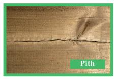
**Pith** is simular to the above defect and quite often found along side each other. Most of this is typically machined to be on the inside of the product.
