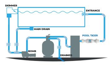
If the return line is too short to install the PoolTiger® inline, a bypass must be performed. Pool Tiger® can be installed horizontally, vertically or diagonally.
