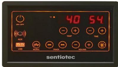
Press **On/off** to switch the control unit on. The heating elements start to heat. The cabin temperature and the operating time are displayed. The time is automatically activated for 60 minutes or to the last selected time. If you press **On/off** again, all functions (heating elements, light and music) are switched off.
