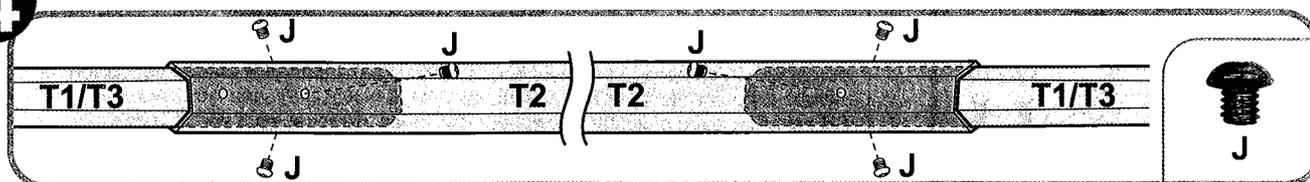
GB To secure the connection of tube "T2" with "T1"/"T3" inside, tighten three screws "J" in the holes on the tube "T2" as shown. (a minimum overlapping of 30cm (11½in) is required).
