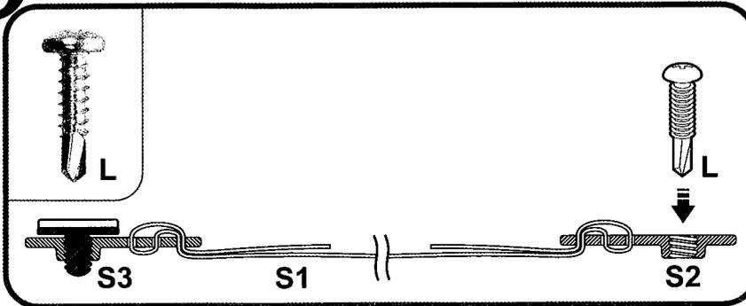
GB Tie "S2" and "S3" on the straps "S1" and use screw "L" to fix "S2" along the tube at even intervals.
