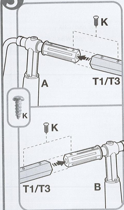
GB **NOTE:** The holes on tubes "T1" or "T3" should be positioned at both ends of the complete tube configuration, ready for connecting the hexagonal tube connectors on "A" & "C". After defining your desired tube configuration, slide the end of preassembled tube sets onto the hexagonal tube connectors on "A" & "C". Make sure the second pre-drilled holes on the tube "T1" or "T3" and hexagonal tube connectors are aligned for screw assembly. Secure the screw assembly with screw "K".
