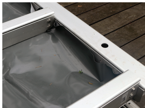
Cleanliness membrane positioned under the casing limiting evaporation
