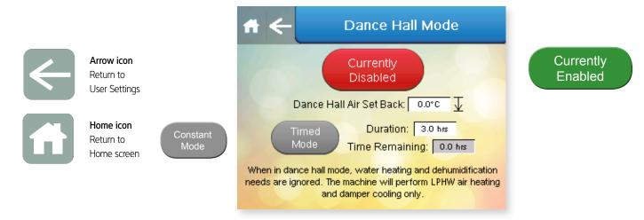
Dance Hall Mode is designed to allow a different air temperature to be used if the pool hall is to be used for a function other than swimming. Water heating and humidity control is deactivated.
