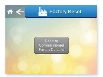
If the settings have been changed in a way that makes the Variheat behave in an unusual way, the original commissioned settings can restored by pressing the Reset to Commissioned Factory Defaults button on this screen. After this has been pressed a confirmation appears, pressing again completes the reset.
