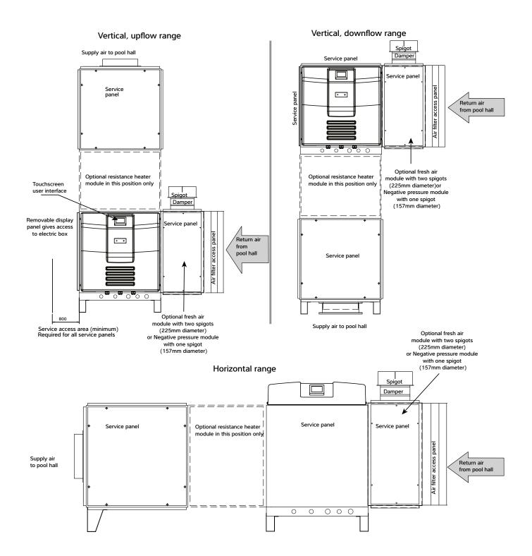
All ambient air ducting should be suitably insulated if plant room temperatures are significantly different from ambient, particularly where the plant room is at pool conditions. Spring return dampers are recommend for exhaust and fresh air ductwork in installations with sub zero ambient temperatures, in case of power failure.
