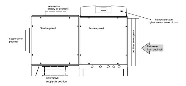
All ambient air ducting should be suitably insulated if plant room temperatures are significantly different from ambient, particularly where the plant room is at pool conditions. Spring return dampers are recommend for exhaust and fresh air ductwork in installations with sub zero ambient temperatures, in case of power failure.
