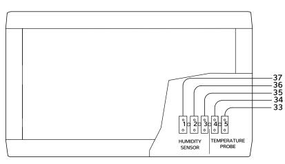
After the Remote Sensor Box has been connected it may be necessary to calibrate the sensor offsets. See Advanced Settings, OFFSETS for how to do this.
