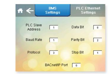
This screen contains settings related to BMS connectivity when using Modbus/ RTU and BACnet MS/TP through the spare RS485 port. The factory default settings are shown. If connecting using BACnet/IP, see the PLC Ethernet Settings screen on page 30.
