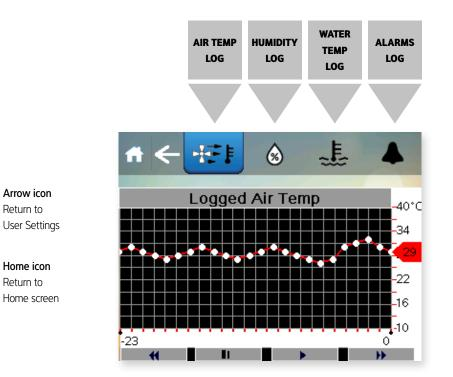
Pressing the buttons brings up a graph of the selected parameter. Choose from Air temperature, Humidity, Water temperature and Alarms. The display is marked up in hours and shows the past 72 hours of activity.
