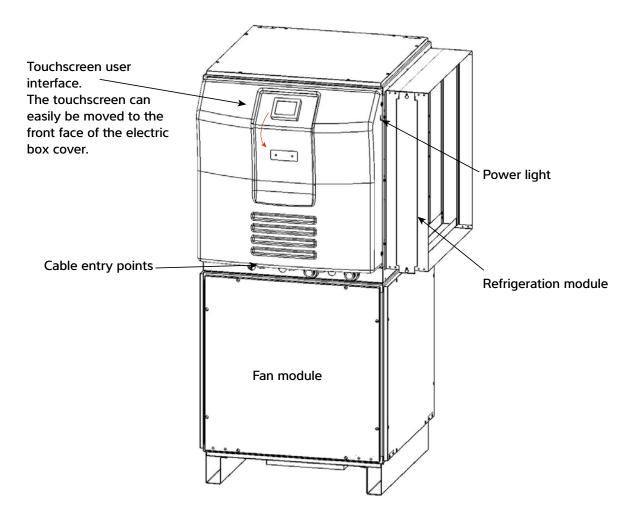
There are 3 cable glands in the electric box tray and two further knock-outs. Use the left hole for access to the power terminals. Use other available access points for the optional interface terminals.
