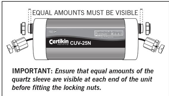
**IMPORTANT: Ensure that equal amounts of the quartz sleeve are visible at each end of the unit before fitting the locking nuts.**
