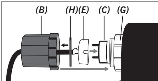
6. Ensure the UV bulb socket is firmly connected to the UV bulb.
