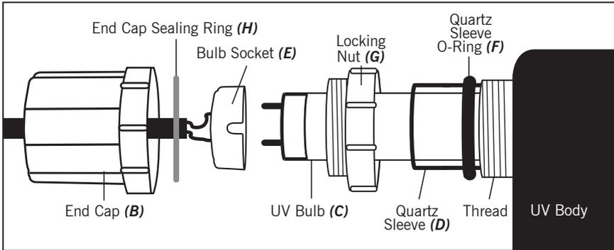
1. Starting at one end of the unit, unscrew the black end cap (B). You will notice that this black end cap houses the bulb socket (E).
