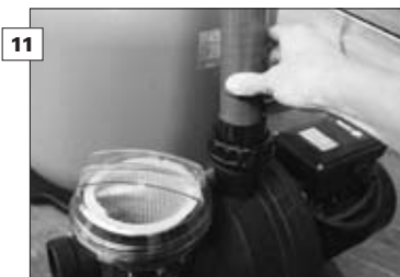
Screw the connector pieces into the filter and the pump. Slide the fittings and the inserts over both ends of the hose. Connect the fittings to the connector pieces, and then tighten the fittings. (see the technical section: 2.4.3 Connections)
