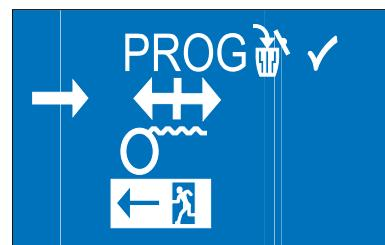
By pressing the middle key “light symbol” shortly the fine tuning is called ( $\leftrightarrow$   $\Rightarrow$  flashes). The Roldeck is in the “CLOSE” position, this indicates that fine tuning is possible for the position “close”.
