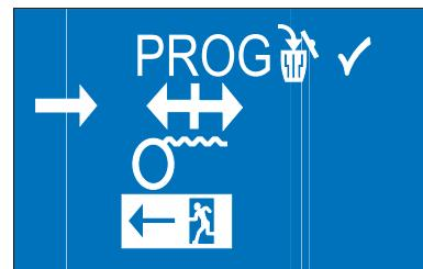
By pressing the middle key “light symbol” shortly the fine tuning is called ( $\leftrightarrow$  flashes). The Roldeck is in the “CLOSE” position, this indicates that fine tuning is possible for the position “close”.
